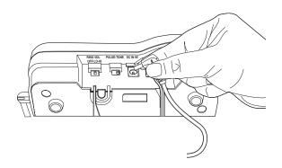
Place the AC Adapter cord inside the molded channel.
